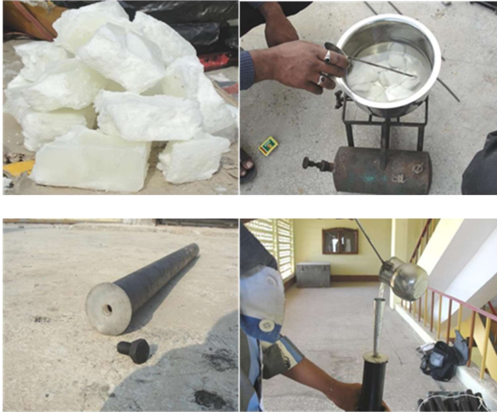
FigA.2: Capsule filling process with paraffin wax
