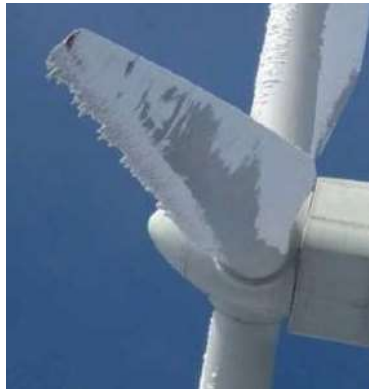
Figure 11. Ice accumulation on wind turbine blades.
