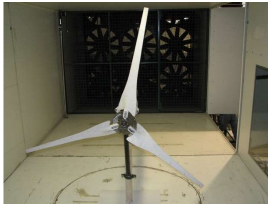
Figure 27. Three-bladed wind turbine
