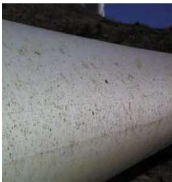
Figure 10. Impact of insects on wind turbine blades.
