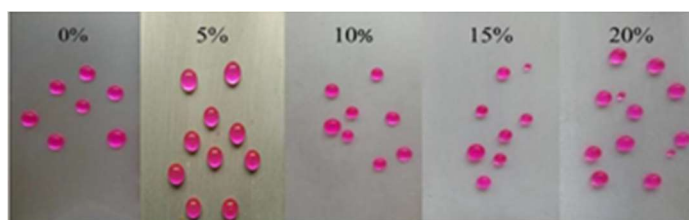
Figure 1. Images of the polyurethane surface modified with SiNPs at different percentages.
