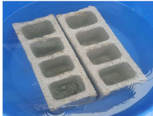
Figure 3. Samples of blocks submerged in water for density and absorption percentage calculation.
