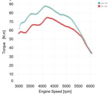
Figure 5 Comparative diagram between torque under H2 enrichment and without H2
