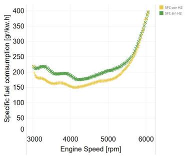
Figure 7 Comparison in fuel consumption under mixture enrichment situation are H2
