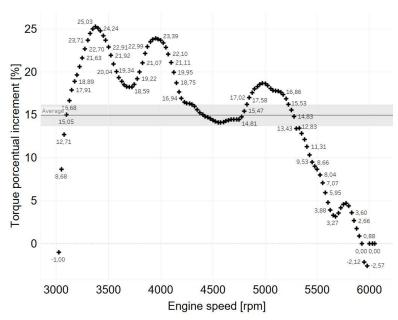
Figure 6 torque with respect to motor speed in H2 increase considerations
