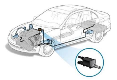
Figure 2. Location of the hydrogen injection valve to the internal combustion engine.
