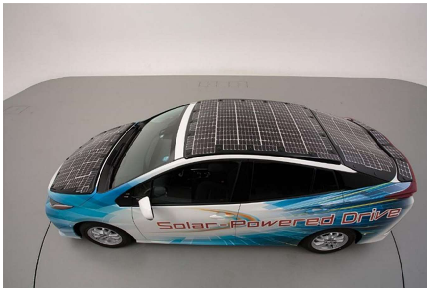
Figure 5. Installed solar skins on a hybrid car. These skins allow for cosmetic customization and cost less than installing regular solar panels on cars [5].
