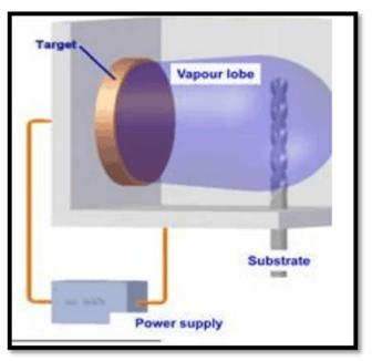
Figure 5: Vapor coating of aluminum (Source: 9).
