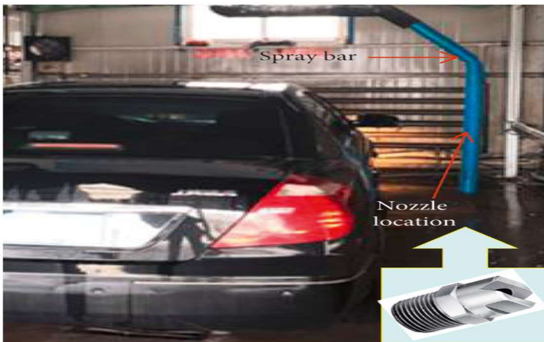
Figure 1 : The physical diagram of the side spray bar of an automatic automobile washer.
